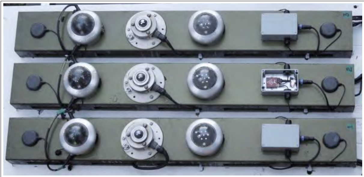
Figure 2: Sensor plates. Three plates mounted on a board for testing. From left to right are GPS antenna B, the shaded SPN, the PIR, the unshaded SPN, the VN300 IMU, and GPS antenna A. On the center plate the VN300 box is open so the IMU is visible.
