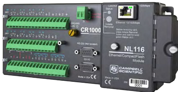
FIGURE 4-1. NL116 attached to a CR1000
