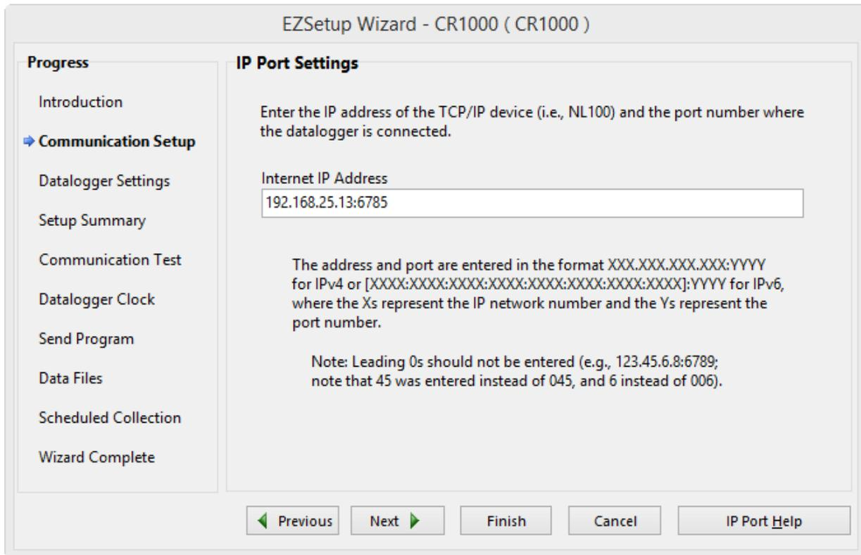
FIGURE 4-5. Setup screen (EZ View) IP Port Settings
