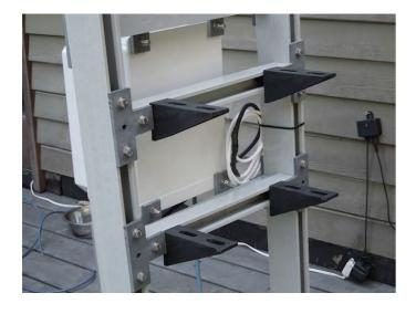
Four triangle brackets can be used to secure the frame to a railing. Heavy duty plastic ties usually work well. Hose clamps or U-bolts can be used for a more secure attachment.
