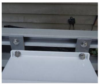
The DAQ electronic box is held by four tabs. It is recommended to leave the tabs on the box and remove from the horizontal struts.
