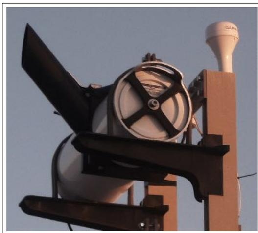
Figure 1: ROSR with rain baffle.
